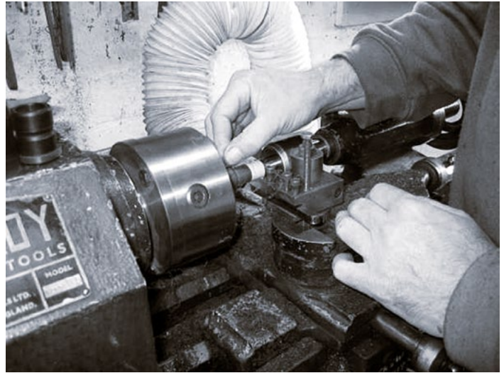
Hazardous exposures are present simply due to the operator's close proximity to the lathe's rotating parts.
