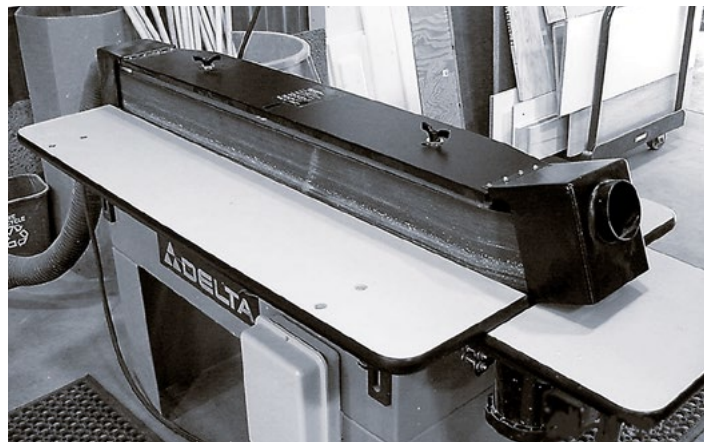
Belt sander missing guards over in-running nip points and belt edge.
