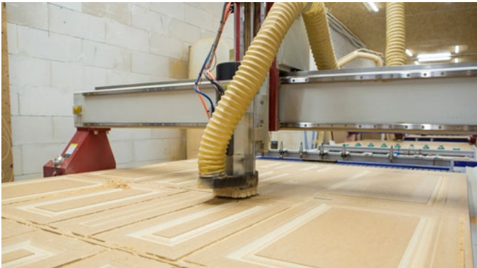
CNC router table equipped with a dust collection system around the cutting tool.
