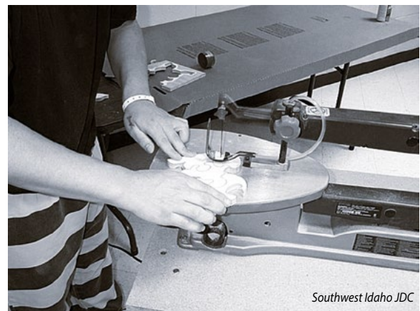
Safety guard/holddown installed.
