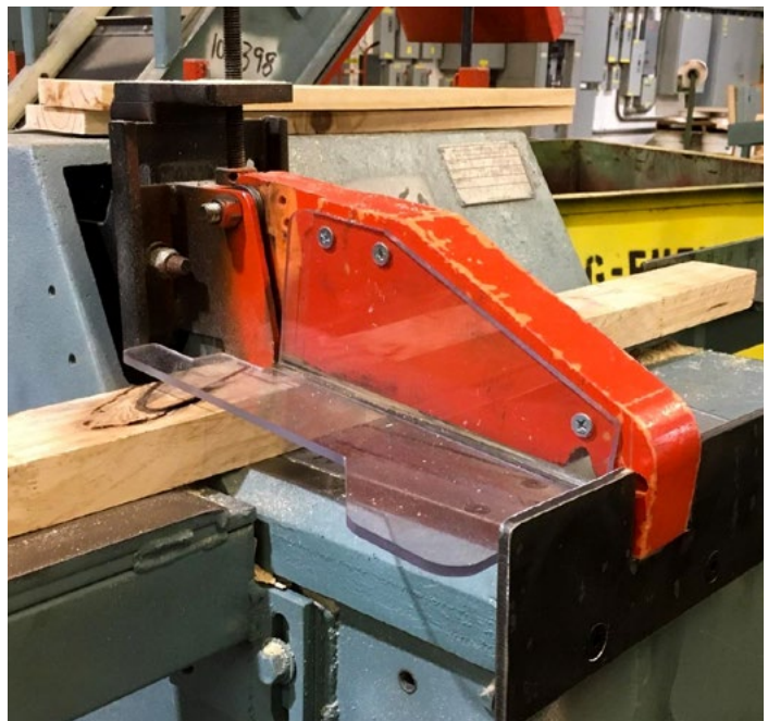
Properly guarded jump saw.
